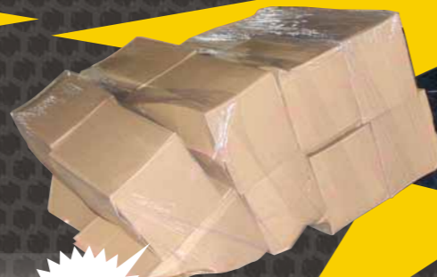
Slipping of plastic pallet when sudden braking
